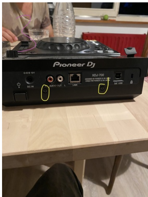
3. Remove two screws and turn the player on its face.
