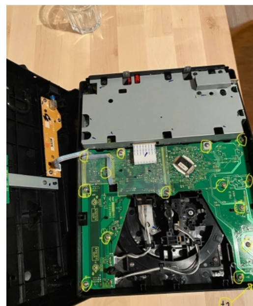
4. Gently open the back, keeping the side with the power button as close as possible to the XDJ body since there's a cable attached. Remove 15 screws.
