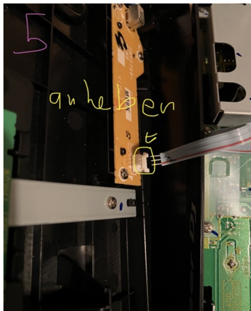
5. Lift up the connector lock (top part of the white plastic), until the cable can be removed without force.
